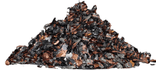
Outputs of shredding process: Copper, aluminum, plastics, iron
